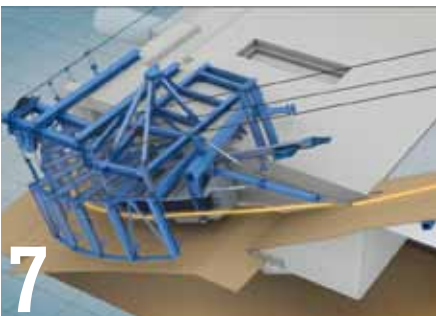
7 Strand is positioned within the cable saddles at the tower and the west end of the SAS
